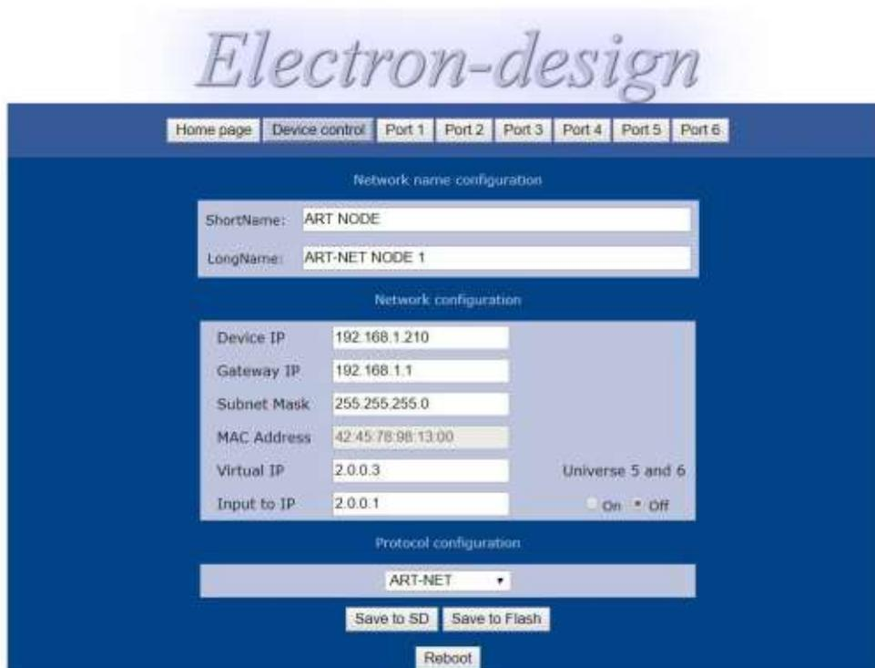
The screenshot shows a web interface for "Electron-design" with a navigation menu at the top: Home page, Device control, Port 1, Port 2, Port 3, Port 4, Port 5, Port 6. The main content area is titled "Network name configuration" and contains two input fields: "ShortName: ART NODE" and "LongName: ART-NET NODE 1". Below this is the "Network configuration" section with a table of settings:
