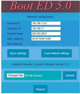
On the boot loader page, you can modify the network configuration, reset all settings to default, and update the firmware to the required version. However, in the boot loader, you can only alter the network configuration.
