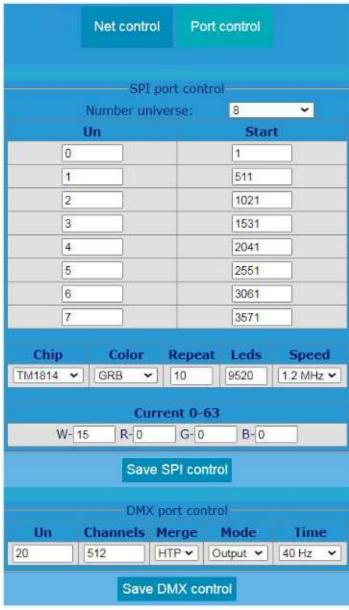
Led port refresh rate. The controller supports increased data transfer rates to the tape. All tested tapes can operate at 1 MHz, however, you must reduce the length of the data wire to 1 meter.
