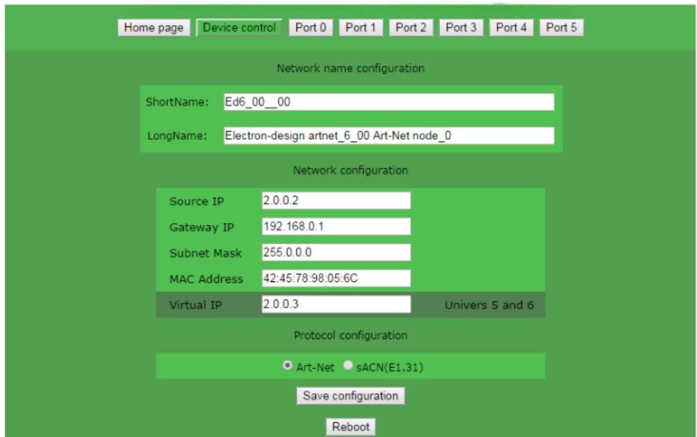
The screenshot shows a web-based configuration interface for a device. At the top, there is a navigation bar with tabs: Home page, Device control (which is selected and highlighted in blue), Port 0, Port 1, Port 2, Port 3, Port 4, and Port 5. Below the navigation bar, there are three main configuration sections:
