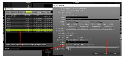
Then click the DMX device, select all the space in the device bar, check the right to enable, send the full frame, and then click the application below, determine.
