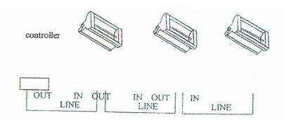
**DMX controller operation** – connect the signal cable according to the chart 2, set the DIP 1 at ON, set the DIP 10 at OFF, set the IP adress, connect to the power, then use the controller adjust the flash speed and brightness of the light. Various strobe connect in a line up to a synchronous effect.
