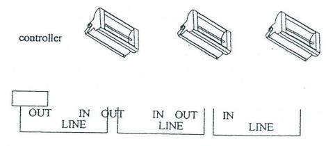
\*Connect the signal cable according to the chart 2 set the DIP 1 at ON, set the DIP 10 at OFF, set the IP code, connect to the power, then, use the controller adjust the flash speed and brightness of the light. Various strobe connect in a line up to a synchronous effect.
